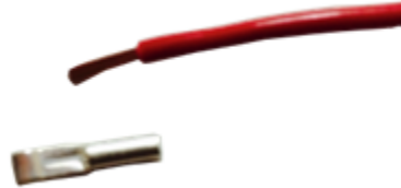
Figure 35: Strip the Wire
