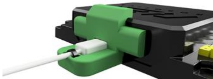
Figure 16: 3D Printed Connector Mount
