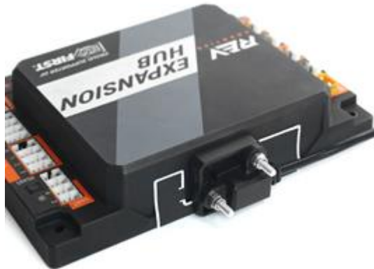
Figure 15: USB Connector Mount
