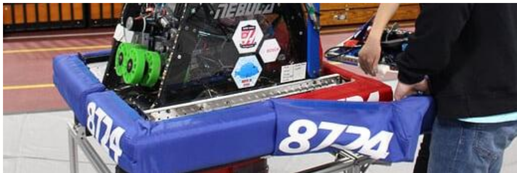
Figure 23: Folding reversible bumper.
