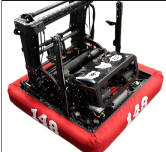
Figure 18: Team #148 with metal frame bumpers.
