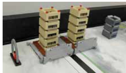
BASE ISOLATION, BUILDING SEGMENTS
