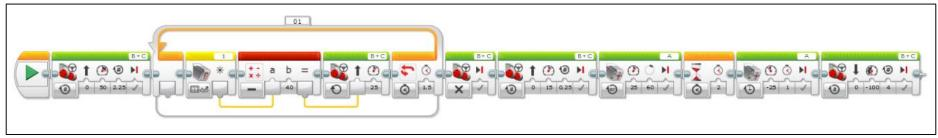
This code will drive the robot out of the Launch area, detect and follow the line directly to the crane, and then activate the lever to drop the blue unit. The red blocks are called 'Math' blocks. You can learn more bout them in Tutorials > Beyond Basics > Math - Basic.
